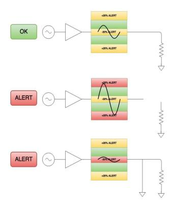
The status of each channel is reported individually via the front panel display - the RS232 port and/or SNMP depending upon the amplifier options selected. The low and high alert limit settings allow the unit to likely detect a failing cable or a disconnected cable condition and will alert the system of a problem.
