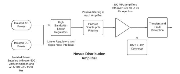
We start off with high-performance switching converters to isolate the unit from the primary power bus and provide the system with a well-regulated DC bus. The converters provide over 500 volts of isolation and feature an MTBF> 150,000 hours (> 17 years). Novus selects all our power converters to be operated at less than 50 % of rated power. Global power and DC power in the range of ±60 Vdc can be used. Power supply redundancy is available
